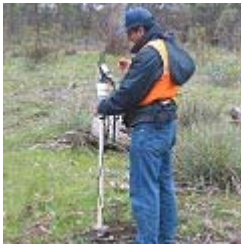
Taking ground measurements of near-surface soil moisture
